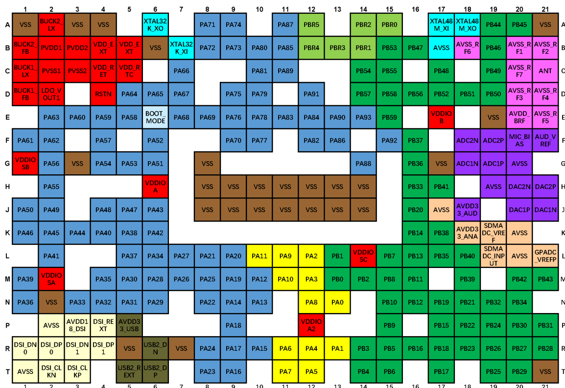
Figure 5-1: SF32LB58x (BGA256) Pin Layout (Top View)
